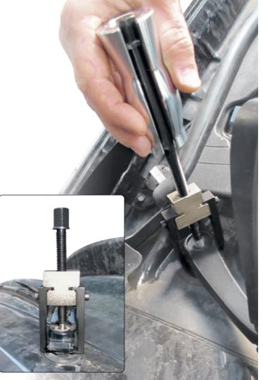
Universal fit for small applications, ranging from 22 - 44mm wide. Ideal also for wiper blades. Brass spindle end cap will prevent damage. Strong enough to even get the toughest wiper arms loose! Ø 22-44mm, depth 30 - 43mm. Kit comes with two sets of adjustable legs.
